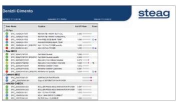
The data management system also contains an MS Excel add-in for direct access to the data stored in SR::x from MS Excel. With this feature, automated reports of relevant operating data that support the operation e.g. as daily and monthly values can be created immediately.
