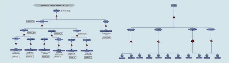
Fault tree with four / two stages and multiple branches
